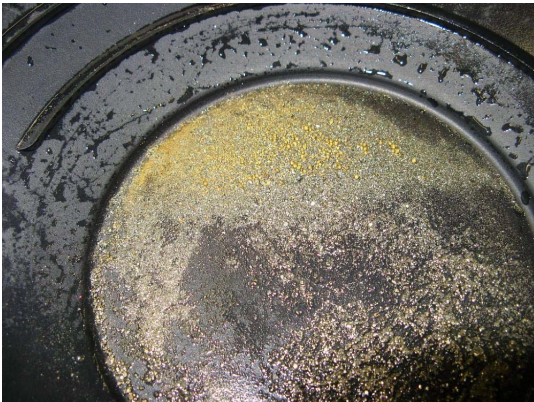
Coarse gold recovered from one of the commissioning samples from the gravity circuit of the A1 sample plant
