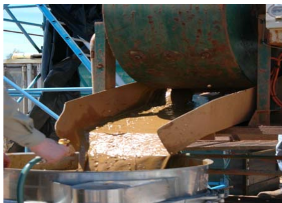
Photograph: Highway sample HWMT03 during pilot-scale scrubbing tests at Oretest. After tumbling in the scrubber for 10 minutes with 50% water, the slurry of nickel bearing clays and coarse rejects are released from the barrel and pass onto the vibrating screen.
