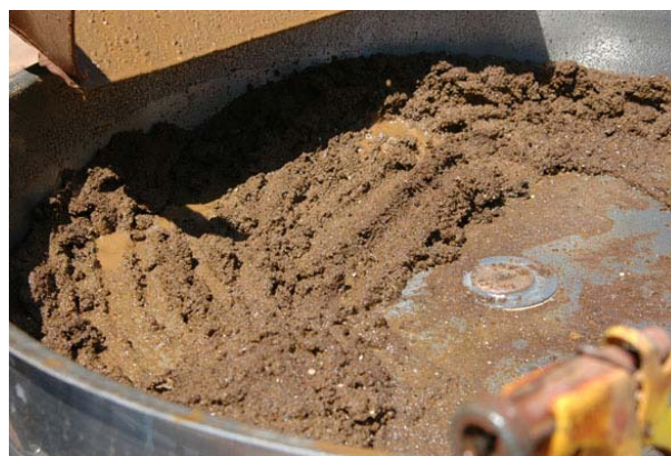
Photograph: The coarse sand like silica reject is clearly visible on the top screen after all the clay bearing ore slurry has washed through the screen.
