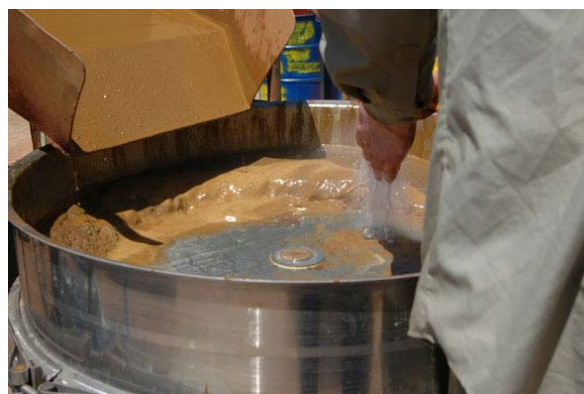
Photograph: The slurry is washed through the screens where the coarse reject remains on the top screen. The separation of slurry and coarse reject is clearly visible on the screen.
