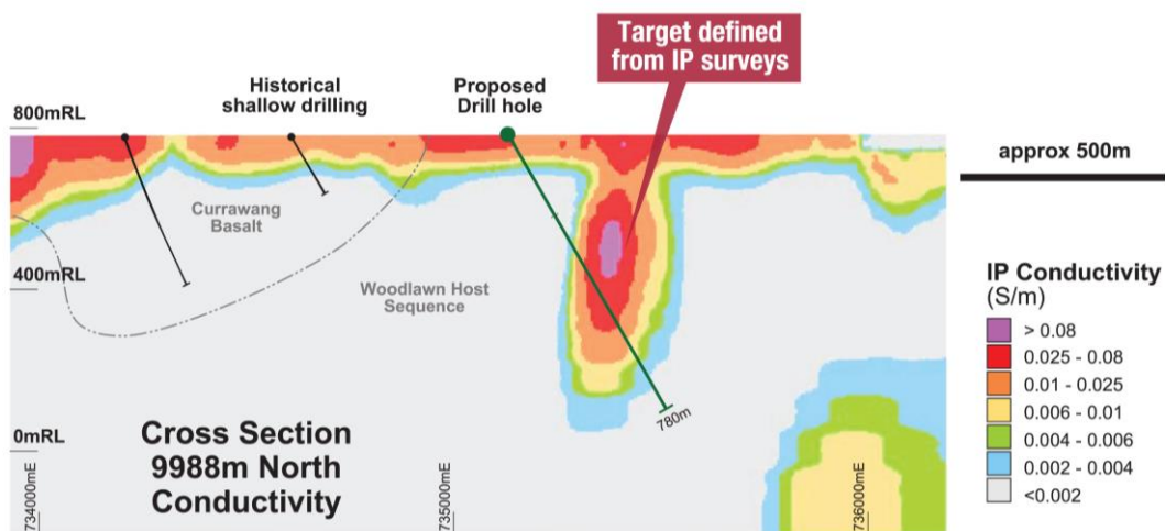
Figure 3: Cross section looking north through the Murphy's prospect showing conductivity response and proposed drill hole.
