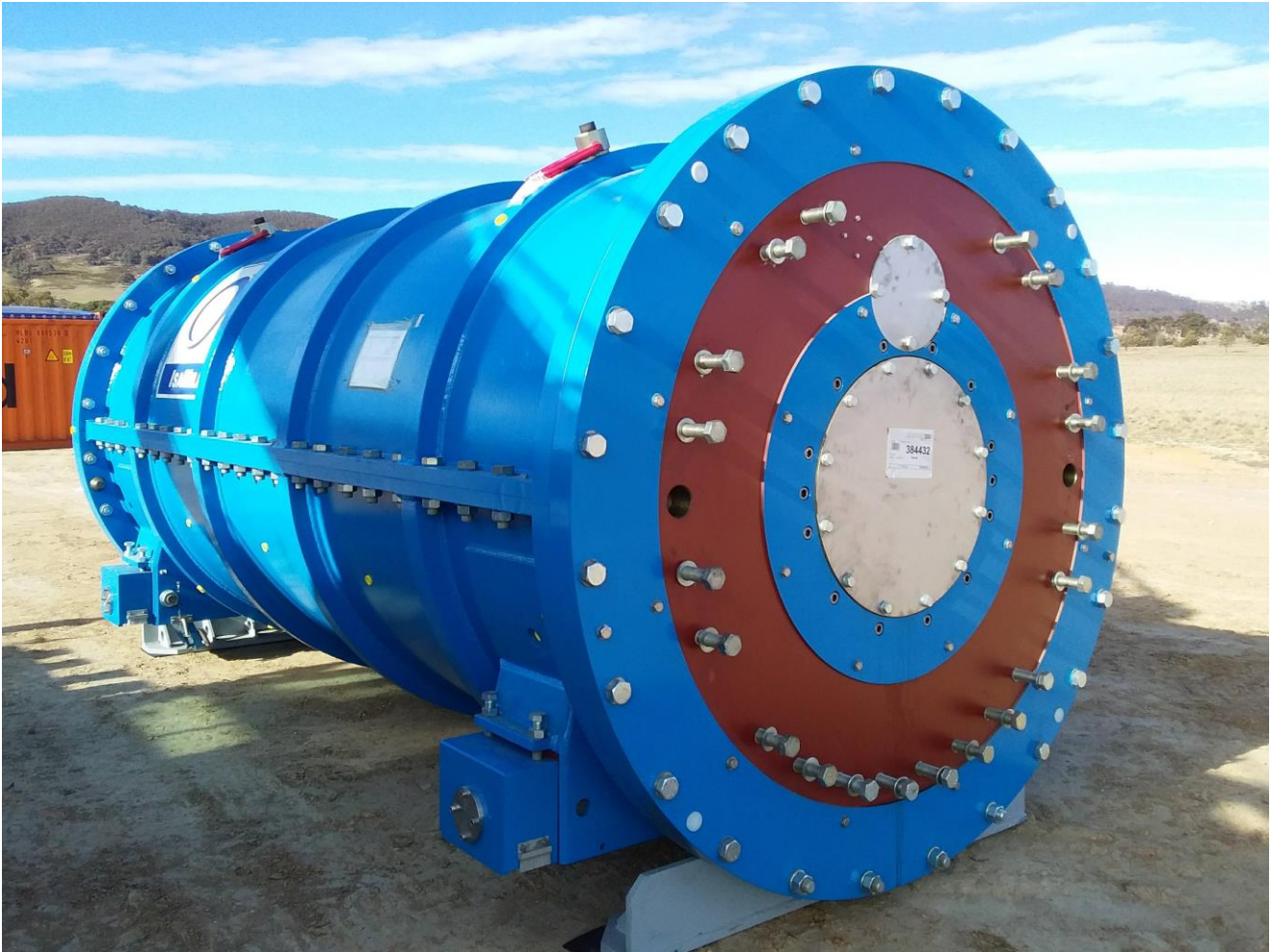
Figure 2: IsaMill ready for installation
