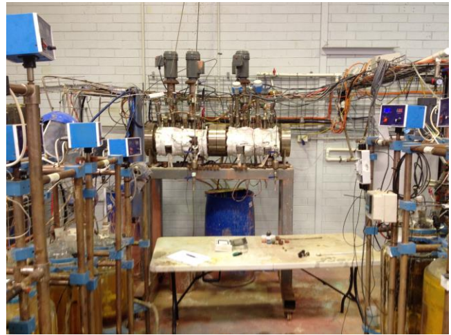
Autoclave used for intermediate stage hydrolysis of iron sulphate for sulphuric acid regeneration. This stage follows the Atmospheric Leach.
