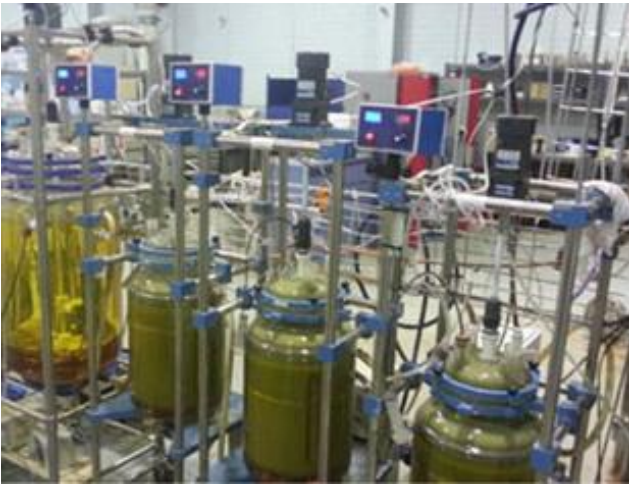
100 litre reaction vessels which form the Atmospheric Leach stage of the flowsheet.
