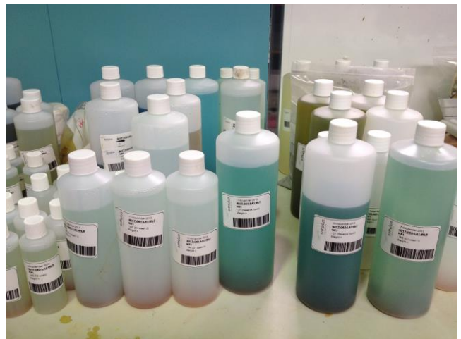
KNP Pregnant Liquor Solution (PLS) following sulphuric acid leaching, purification and acid recovery, from which Mixed Hydroxide Product can be crystallized. The distinctive green coloration in the PLS samples reflects the amount of nickel in solution.
