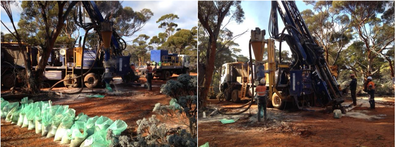
Figure 2 Recently commenced Bedonia RC drilling – Figure 3 Bedonia RC drilling initially testing the magnetic anomaly
