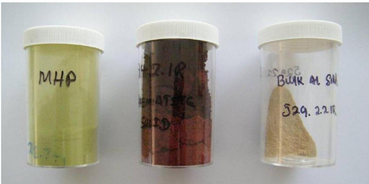
*Heron's first KNP nickel production, from left to right green nickel MHP assaying 40% nickel, dark red hematite assaying 56.6% iron and grey-yellow aluminium hydroxide assaying 20.6 % aluminium*
