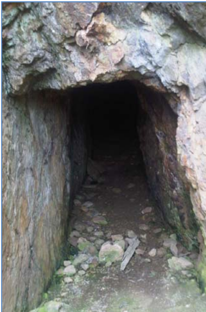
Figure 7 Photo of historical copper workings shaft at Califat. Green colouration is largely related to the secondary copper mineralisation malachite. Opening ~ 1.5m high
