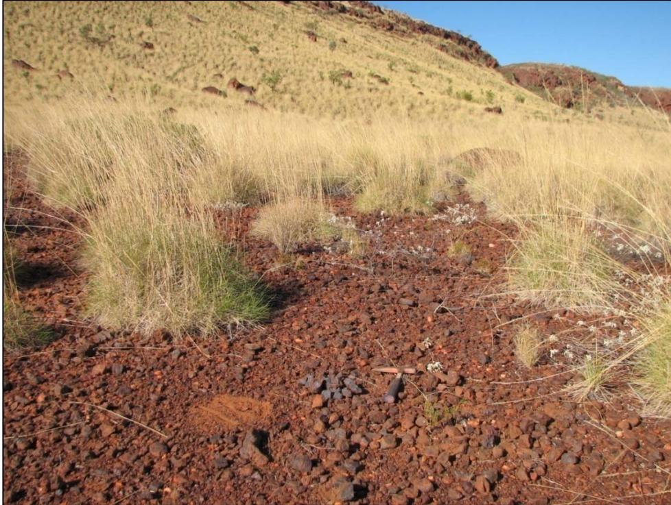
Figure 7 Detail of material from sample location SG05 showing dominantly good quality iron-ore fragments
