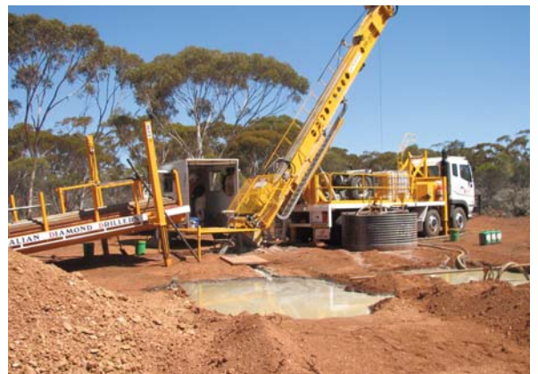
Diamond drill rig drilling for nickel sulphides at Avoca Downs and Kalpini
