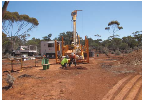
Diamond drill rig drilling for nickel sulphides at Avoca Downs and Kalpini
