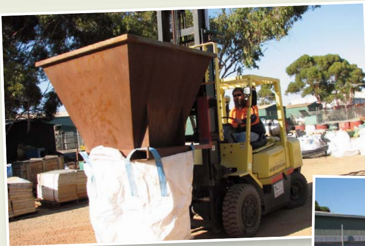
John Briant (Field Supervisor), uses his superior fork lifting skills to show the technique used to obtain bulk samples of ore to ship to China.
