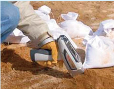
Above: The Niton XRF Analyser at work in the field
