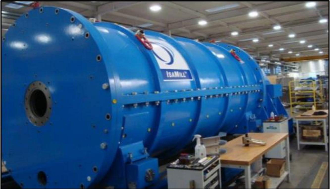
Figure 6: Woodlawn's IsaMill M10000 shell – original critical path item that is ahead of the forecast fabrication schedule.
